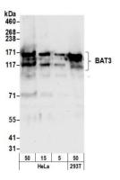
Detection of human BAT3 by western blot. Samples: Nuclear extract from HeLa and HEK293T cells. Antibody: Affinity purified rabbit anti-BAT3 antibody A302-038A (lot A302-038A-2) used for WB at 0.04  $\mu$ g/ml. Detection: Chemiluminescence with an exposure time of 10 seconds.
