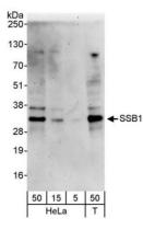
**Detection of human SSB1 by western blot.** *Samples:* Whole cell lysate from HeLa (5, 15, and 50 µg) and HEK293T (T; 50 µg) cells. *Antibody:* Affinity purified rabbit anti-SSB1 antibody A301–938A–M used at 1:1000. *Detection:* Chemiluminescence with an exposure time of 3 minutes.
